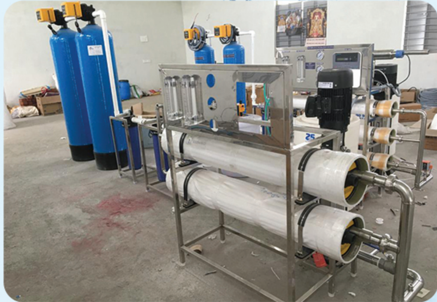
2000LPH Fully Automatic Membrane Filtration System
