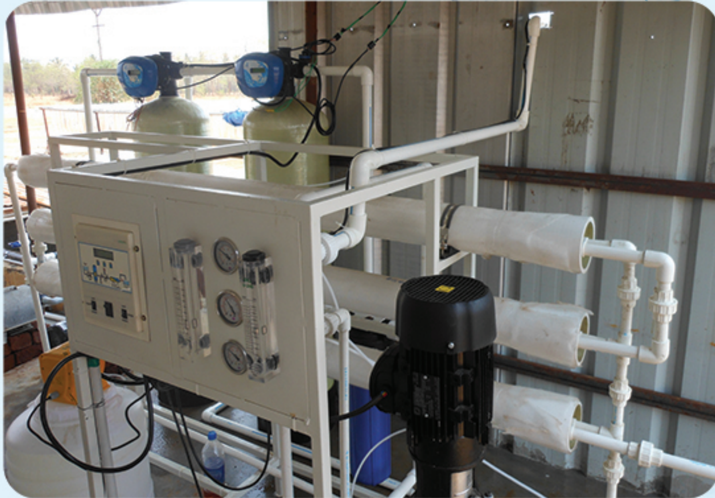
1200LPH (Automatic operated membrane filtration system with pressure sand filter, Activated carbon filter, backwash and rinse water recycle system)
