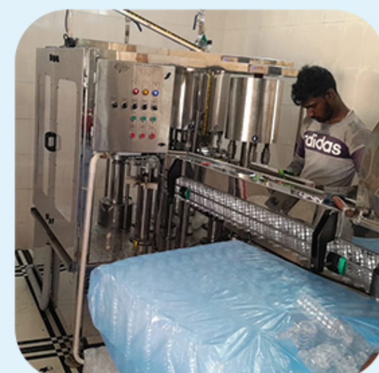
PET Bottle Rinsing, Filling, Capping, Batch Coding and Web Seal Packing Machine
