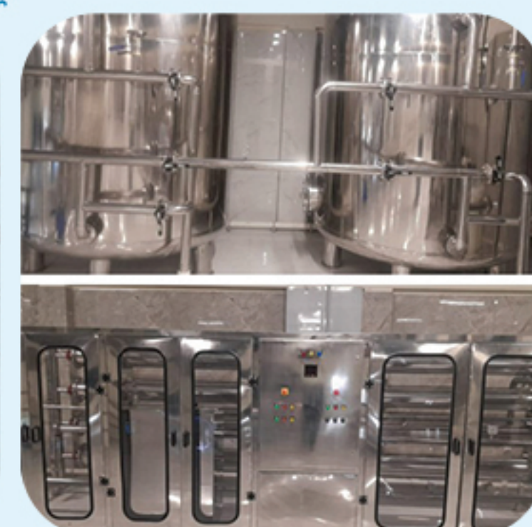
20000LPH (Fully SS 304 Membrane Filtration System)
