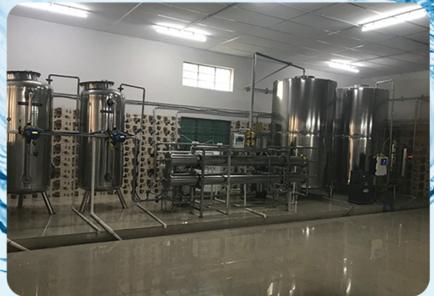
6000LPH (Fully SS304 automatic Membrane Filtration System with storage tank, post filtration, UV and Ozone generator with oxygen concentrator disinfection system)
